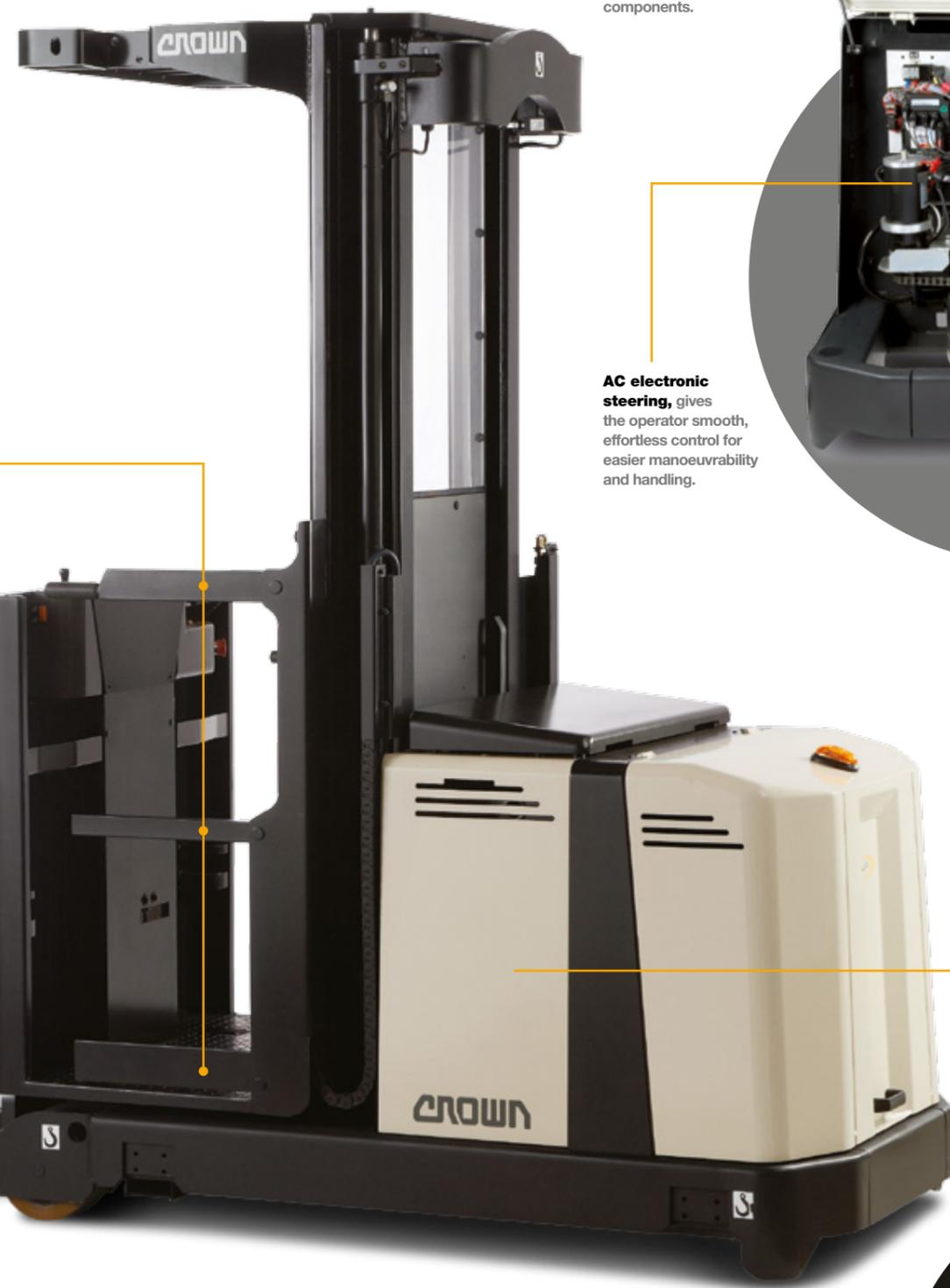
**Simplified service** results from a large hinged cover for easily accessible internal components.
