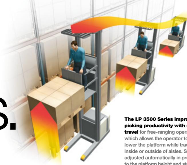
The LP 3500 Series improves picking productivity with diagonal travel for free-ranging operations, which allows the operator to lift or lower the platform while travelling inside or outside of aisles. Speed is adjusted automatically in proportion to the platform height and steer angle.
