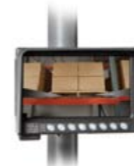
Mast mounted camera with colour monitor
